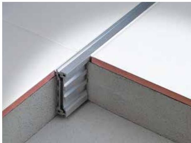
COFLEX CK technical sliding expansion joints are conceived for thin-set installations. Two metal sides interlock and slide with an internal gap of +/- 2mm, redistributing differential movement due to material compression and expansion. The profile comes assembled in a "neutral" position, held together by an elastic gasket in the lower profile section. It offers durability and high resistance to vertical loads with a modern design. Suggested floor bays: 16 - 25m<sup>2</sup>.
